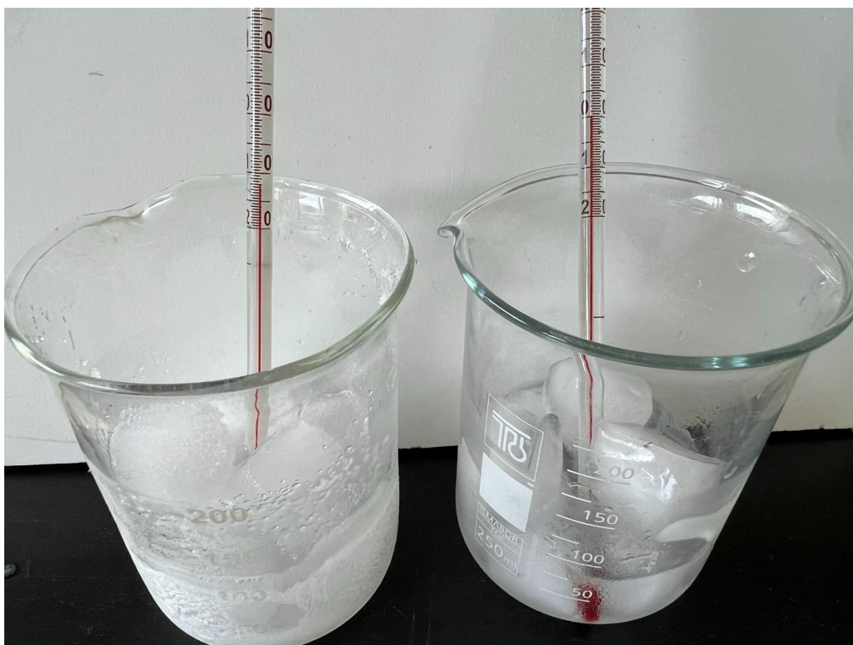
Left: Ice cubes with salt. Thermometer indicates more than 10°C below zero. Right: Regular ice cubes. Thermometer indicates the regular melting temperature of water 0°C.
